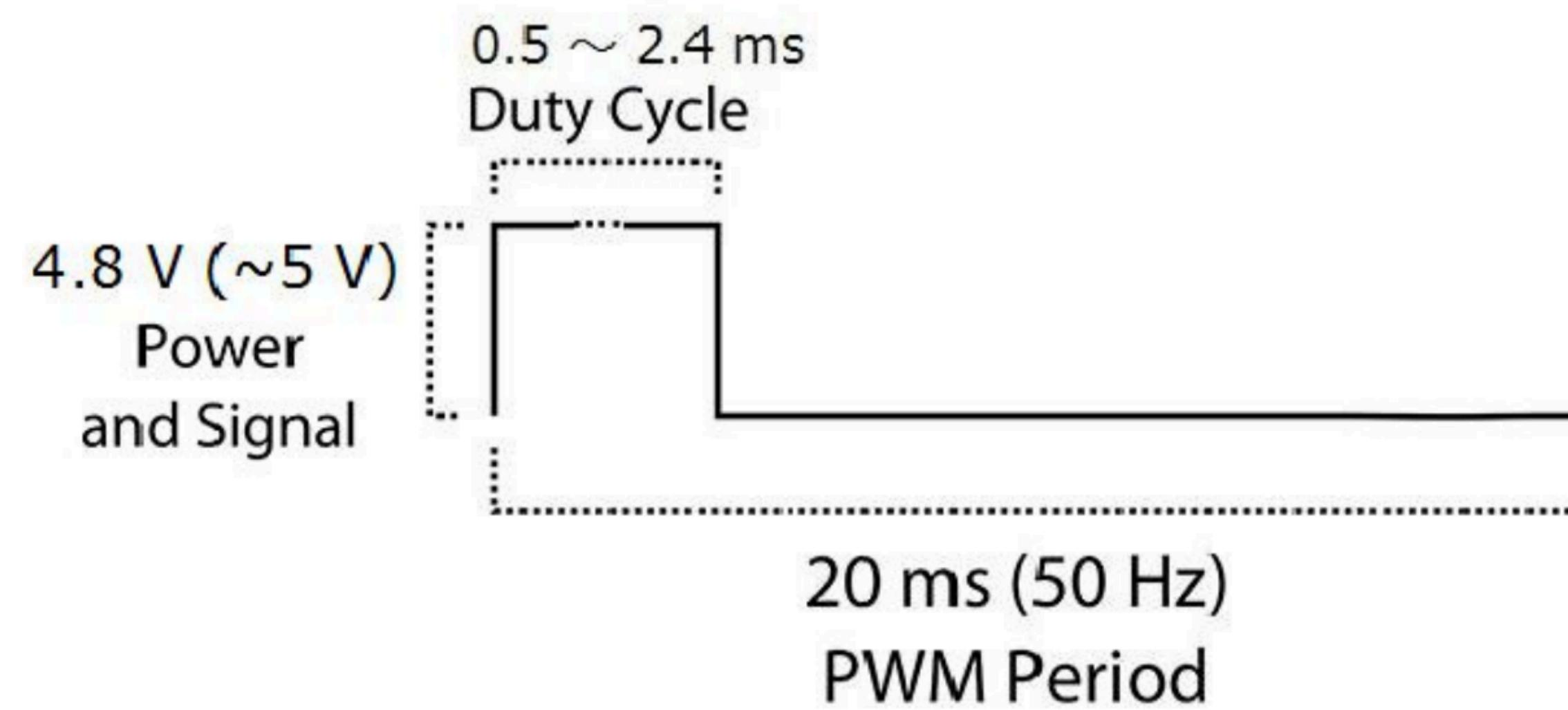
Position "0" (1.45 ms pulse) is middle, "90" (~2.4 ms pulse) is all the way to the right, "-90" (~ 0.5 ms pulse) is all the way left.
